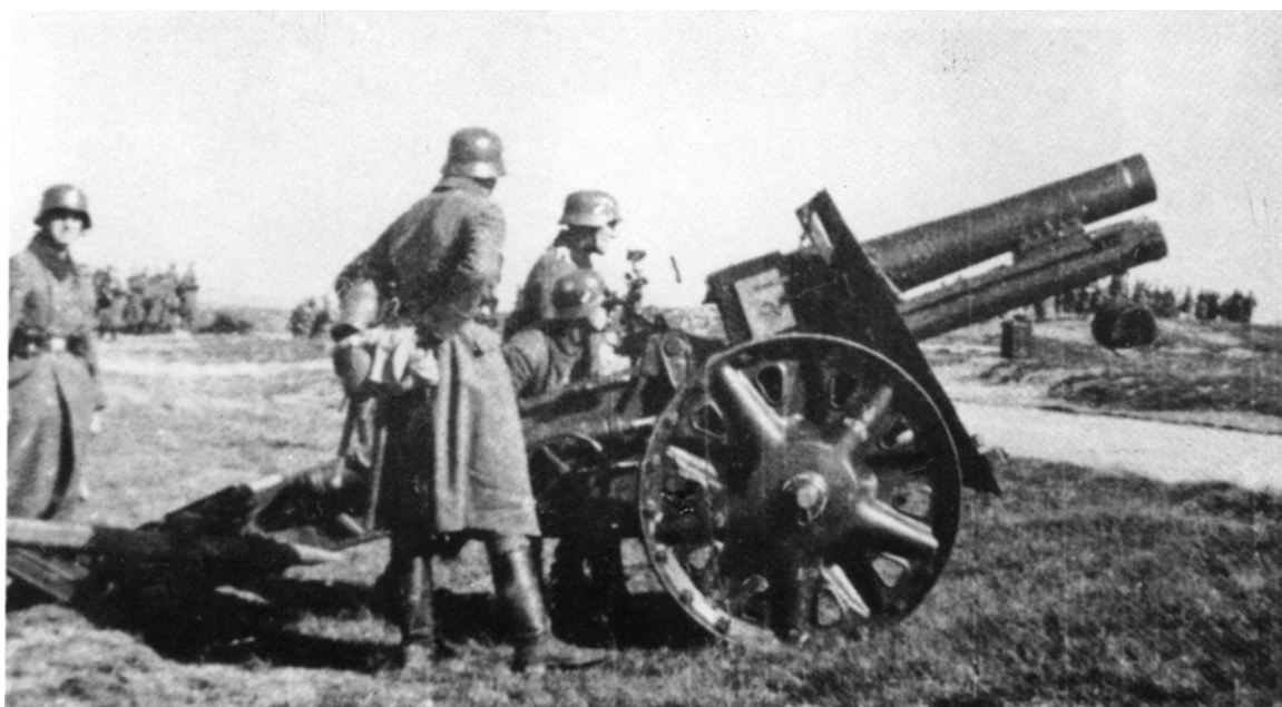
A heavy infantry gun in firing position, being aimed with a panoramic scope.
